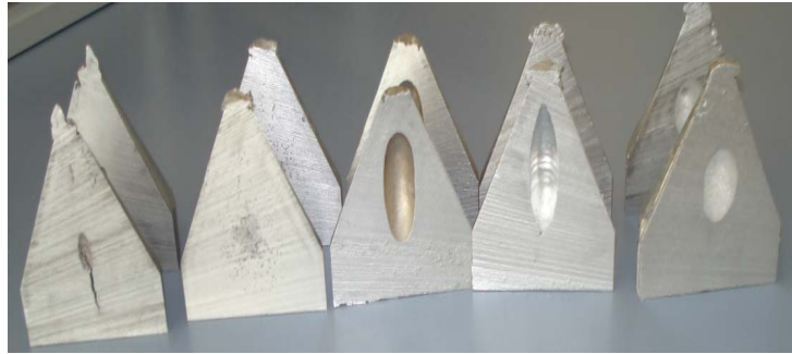
Fig. 7. Typical shrinkage porosity obtained using Tatur test.
