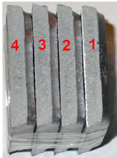
Fig. 5. Fractured pieces of K-mold test sample.
